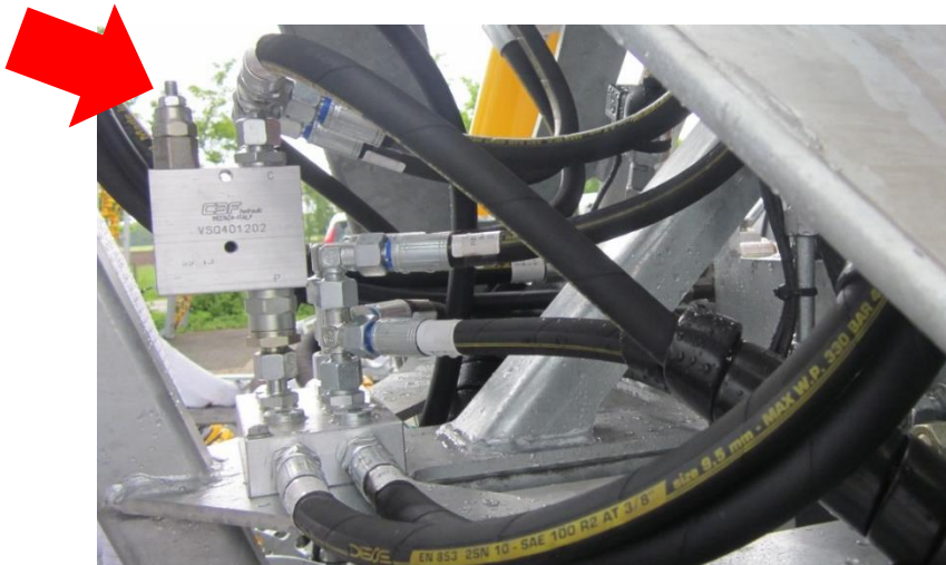
Setting sequence locking hooks, this is set at the factory.
